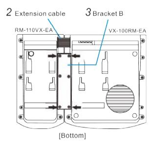
**Step 4.** Using the 8 screws provided (follow shown in the picture) and two junction bracket A to secure two units.
