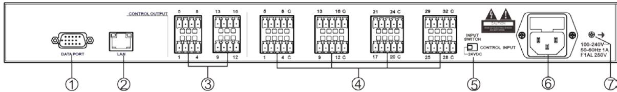
①DATA PORT: data upgrade interface, it's used for firmware upgrade.
