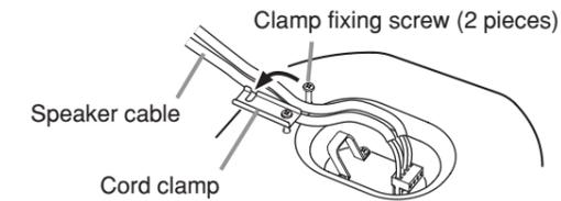
**Tighten the clamp fixing screw to fix the speaker cable with the cord clamp.**
