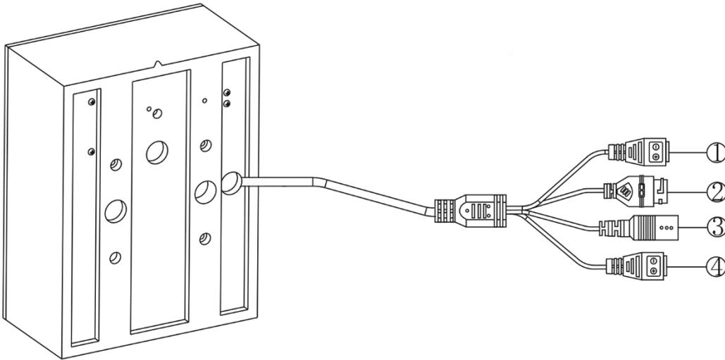
① Amplifier output connector: connector color is black, specification is 3.81-2P, connecting external speaker, when the speaker receives the broadcasting, the same sound can be heard from the speaker. The Rated impedance:  $8\Omega$ , the rated output power: 10W
