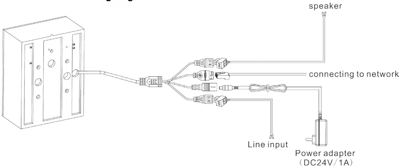
Note: 2P green connector is for line input, 2P black connector is for amplifier output.
